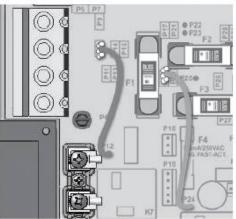
Note: To convert model to a 120 V system, the white (common) accessory wire must be moved. See wiring diagram for details.
