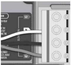
Connections for 120 V heaters (1 kW)
