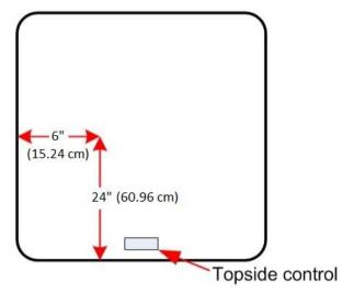
FIGURE 1: ELECTRICAL CONDUIT LOCATION
