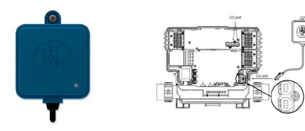
The in. touch 2 spa transmitter must be installed under the spa skirt, at least 12" (30 cm) away from any metal component or structure, as close as possible to the house to optimize the signal strength.
